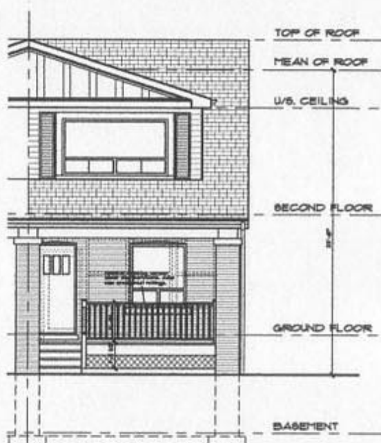
PROPOSED FRONT (NORTH) ELEVATION. Scale = 1/4" = 1'-0".
